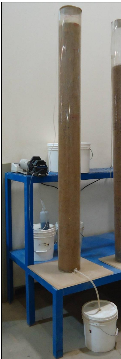
Figure 6-2. ODAS/Stratex Project Column Leach Test Apparatus
